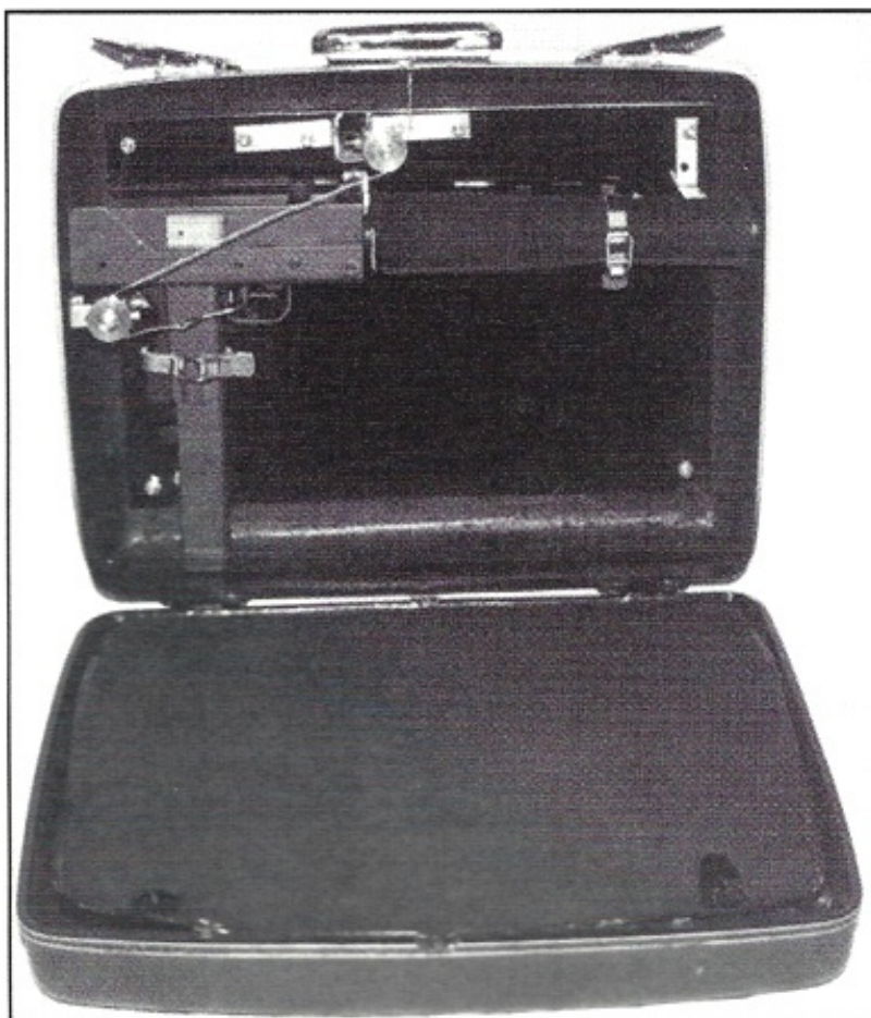
Left: MAC 10/45 operational briefcase made by the author. This operational briefcase houses a M10/45 which is held in place by two brackets. The trigger is actuated by a wire pulley system which exits the top of the case near the handle. The suppressor end cap is screwed through the case from the outside to help secure the M10.
