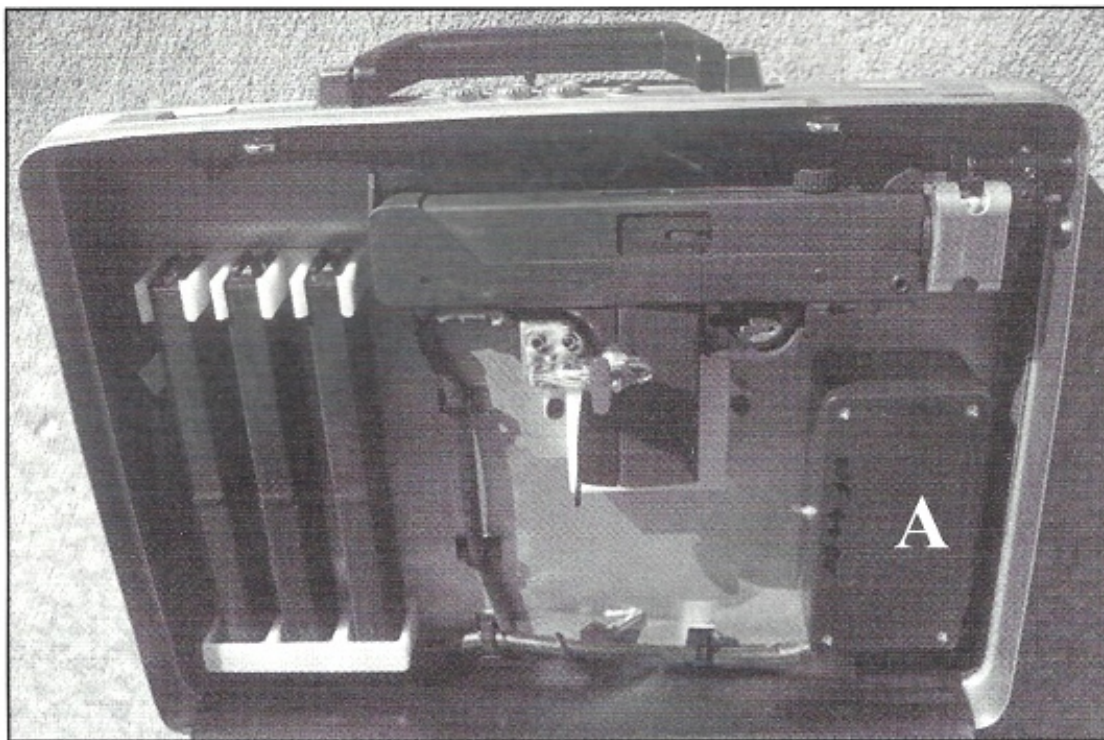
Left: DAW Operational briefcase internals. The SWD M11/9 is held in place by a front block and a clamp on the magazine well. The box on the lower right (A) holds the battery. There is a button on the side of the box that will turn off the circuits from the inside. Teflon blocks on the right hold three magazines.
