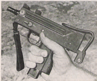
With its 16-round magazine in place and wire stock folded and telescoped, the M-11 is not much larger than ordinary handgun. Carrying strap aids in controlling it on full-auto.
