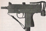
Fire selector is on left side of both M-11, above, and M-10 and must be pivoted in half-circle to change from semi to full-auto.
