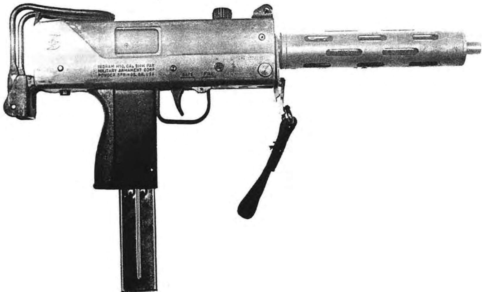
MAC 10 WITH ALTERNATE TUBULAR BARREL EXTENSION FITTED
