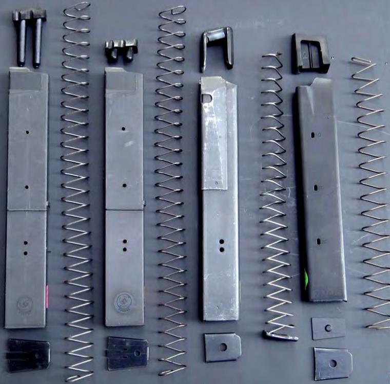
Note: both Zytels show non-standard witness holes that I drilled in sides of magazine.
